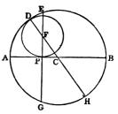
Now, EF. FG = DF. FH (xxxv.), and  $PF^2 = DF^2$ . Hence, by addition, making use of II. v., and II. iii..  $EP^2 = DF$ . DH = twice rectangle contained by theradii.
